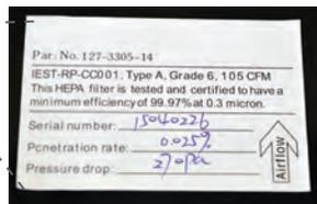
The HEPA filter is individually tested and certified to be 99.97% efficient at .3 microns according to IEST-RP-CC001 test requirement.
